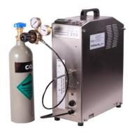
VC - Aero 5000 and 1300 - These generators produced an aerosol to EN-ISO 14644-3 for filter testing applications, They are available in a number of configurations, at outputs to suit small to large scale air flows. The particle size remains extremely consistent across the entire range. These units will support Emery 3004, Durasyn 164, Concept Smoke Oil 135 (identical equivalent to Ondina EL), Ondina 919.
